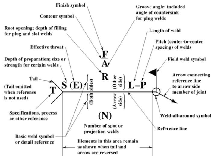
Since, the symbol is above the reference line, then the weld occurs on the “other side”. Also the length of the weld is shown in between the weld symbol and the arrow as 2”. The second number, 6” refers to the center to center spacing of the welds. The number between the tail and the weld symbol describes the depth of the weld. Finally, the weld symbol is a square weld.
