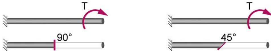
Figure 12: Ductile materials (left) will flex in torsion, until the maximum shear stress is met and the material will fail at a near 90 degree angle. Brittle materials (right) will not flex in torsion and will fail in tension at an angle near 45 degrees to the longitudinal direction.
